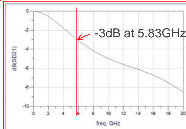
Figure 27 HS-G4 Reference Package Insertion Loss Information
